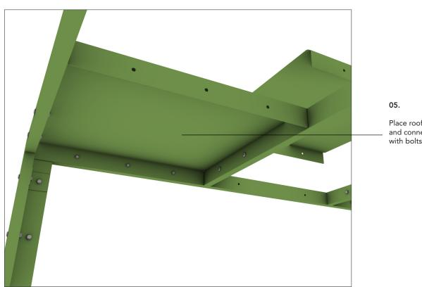
Place roof segments as shown and connect to the beams with bolts.
