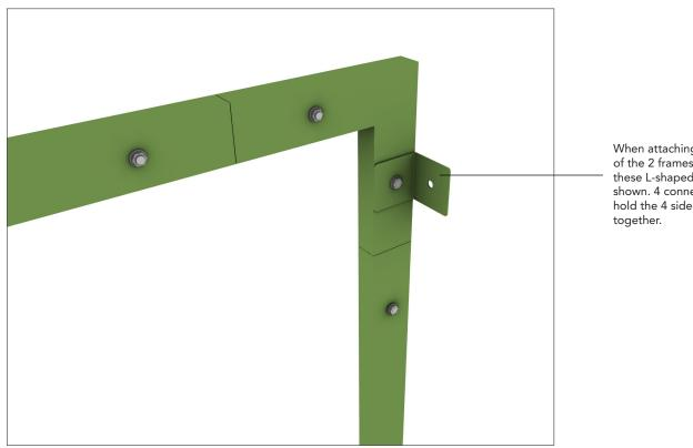
When attaching the leg posts of the 2 frames, connect also these L-shaped connectors as shown. 4 connectors that will hold the 4 sided structure
